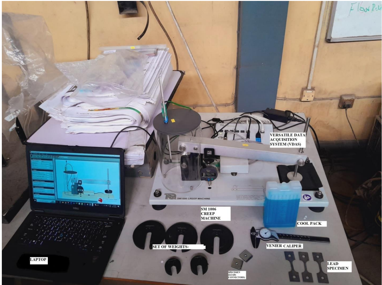
Fig 2.1 Complete display of system, Materials and equipment
